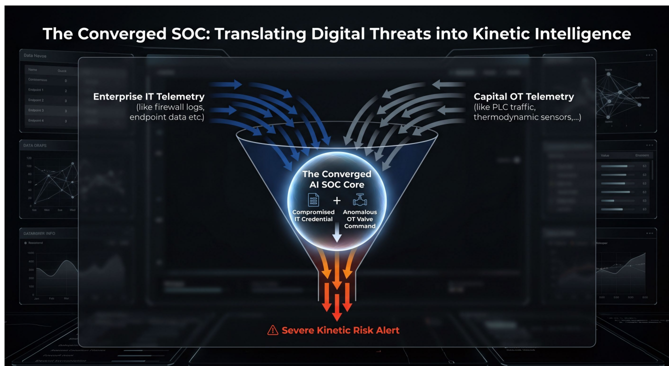
Figure 7. The Converged SOC Architecture. Illustrating the synthesis of Enterprise IT network data and Capital OT physical telemetry. By funneling these disparate streams into a unified AI correlation engine governed by frameworks such as MITRE ATT&CK for ICS, the SOC translates isolated digital anomalies (e.g., stolen credentials) and physical deviations (e.g., erratic valve commands) into actionable, high-severity kinetic risk alerts before mechanical failure occurs.
